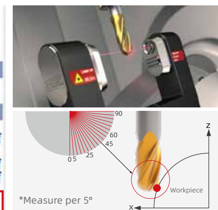
Inspect Tool Contour on the Machine
