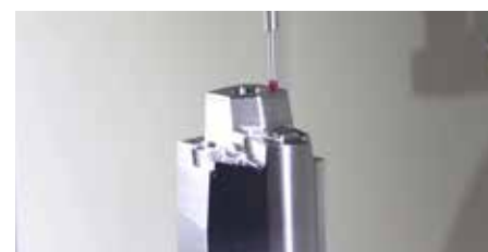
02-Obtain Actual Position on the Machine
