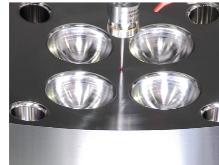
Inspect the Remaining Stock on the Machine
