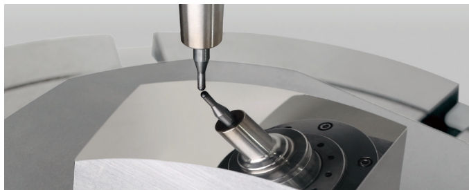
0.1 \mu\text{m} Feed, 1 \mu\text{m} Cutting
