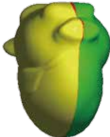
Parting Painting for 3D Model
